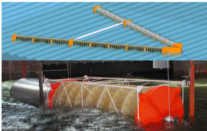
Figure 1: Illustration of the full scale design (top figure) in 2007 and the test model (bottom figure), which represented a scaled section of one of the legs.
