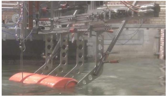
Figure 6: The PTO test model, where the new design of the PTO was tested and optimized.
