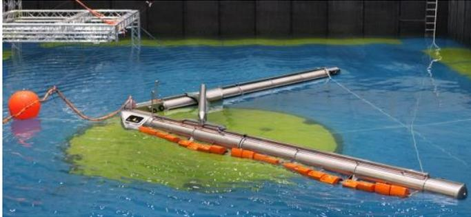
Figure 4: The first complete model that was tested in the CCOB test facilities in Santander (Spain).
