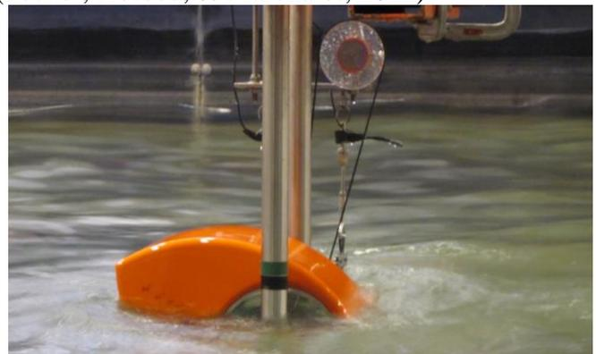
Figure 3: Picture of the model with one rotor, which was mainly used to benchmark its power production capabilities, and to optimize its weight distribution and PTO control.
