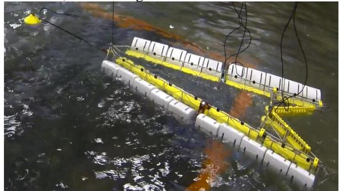
Figure 7: The second full model, representing the new structural design and resulting in a reliable mooring design.
