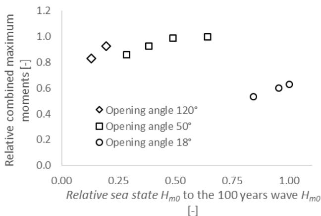
Figure 9: The relative maximum combined bending moments in the middle of a leg of the structure against the relative significant wave height (Pecher & Kofoed, 2014).
