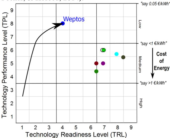
Figure 11: The development trajectory of the Weptos WEC, together with the current estimated TRL-TPL of some of the leading wave energy technologies.
