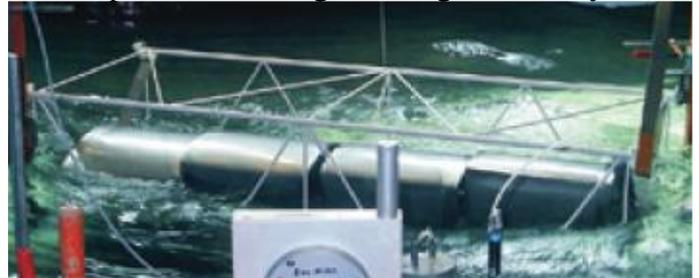
Figure 2: The first model containing Salter’s duck inspired rotors and a very simple Coulomb type PTO system based on a ratchet mechanism between the rotors and the common axle.
